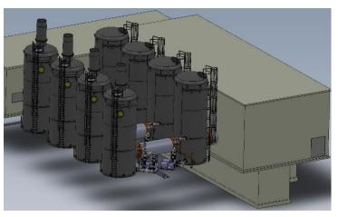
Because of the high H2S concentration in the foul air, Ipec designed a two-stage chemical scrubber system with a total capacity of 300 000 m³/hour. The system exists out of four trains each individually treating a flow of 75 000 m³/hour. Each train holds a stainless steel fan connected to a suction manifold for air extraction from the different locations inside the pumping station. Each fan is provided with a pressure transmitter and flow sensor to control the flow by VFD.
