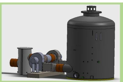
3D-model of odour control unit, University of the Philippines Skid assembled unit
