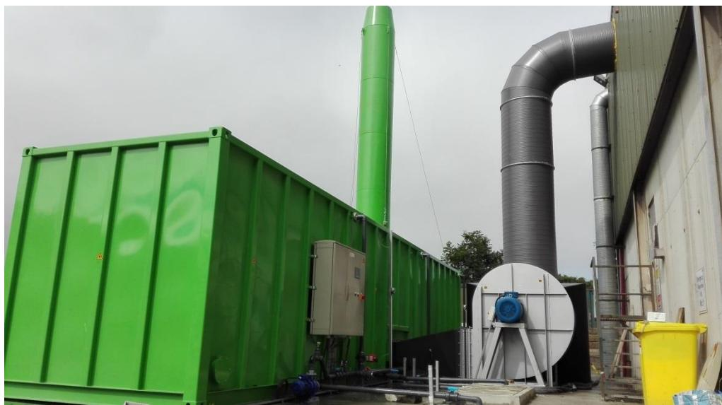
The system is custom made, based on the size of the process hall and the odour load. It can be provided in 1 container processing a flow up to 70 000 m<sup>3</sup>/hour. Depending on the requirements, it can be highly automated and provided with SCADA or other controls which make the system easy to operate.
